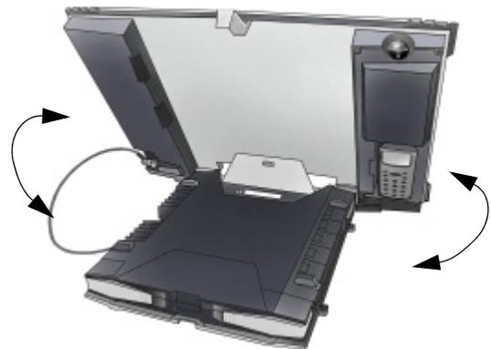
2. Tilt the antennaEXPLORER 700 slowly up or down until it points in the correct vertical direction, known as the **Elevation**. Hold the transport lock and the support bracket while moving the antenna. Do not place your hands on the antenna.
