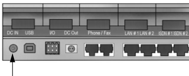
**Connecting to a 100-240 V AC electrical outlet:** Connect the AC/DC adapter to the DC Power input on the side of the EXPLORER 700. Then connect the power cable between the 100-240 V AC electrical outlet and the AC/DC adapter.
