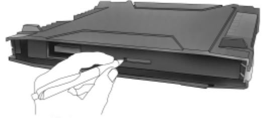
2. Take the SIM card holder out and place the SIM card in the holder, with the printed side visible.
