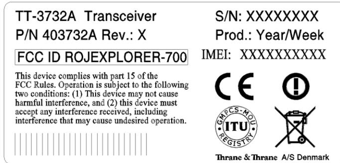
The following label is placed on the antenna part of the EXPLORER 700.
