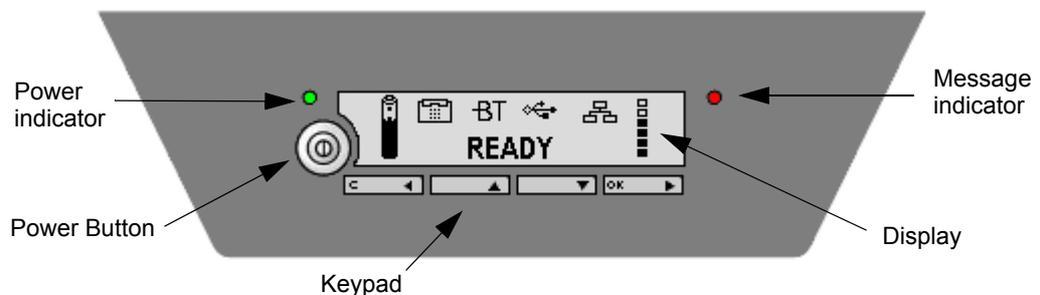
For information on how to use the keypad and display, and for an overview of the display menu system, see *Using the display and keypad* on page 35.
