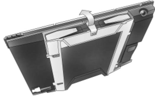
2. You can now flip up the antenna module and access the keypad and connectors on the EXPLORER 700.
