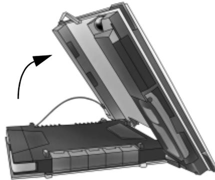
2. Gently lift the transceiver out of the antenna frame.
